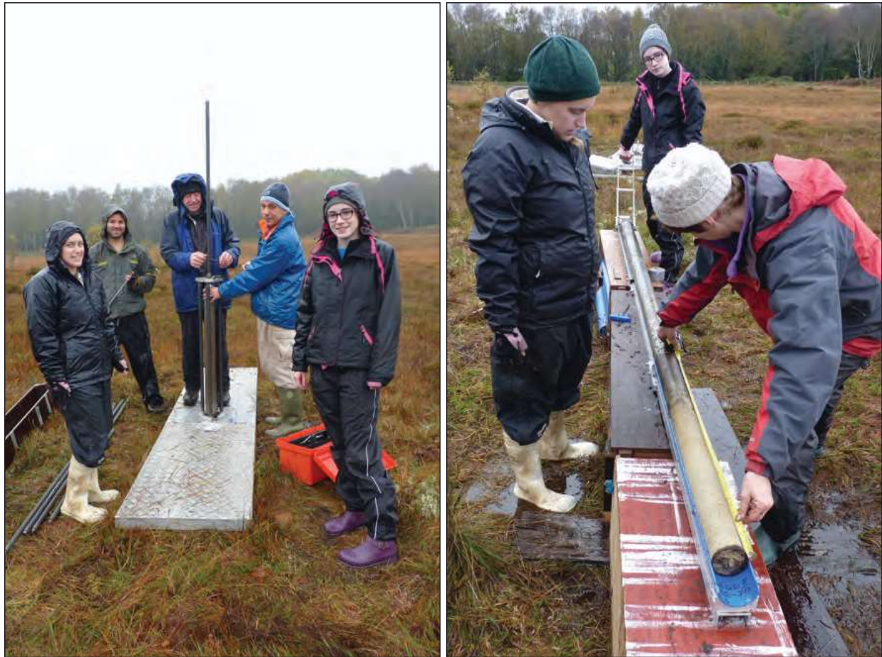
Illus. 3.3—(Left) Coring team members Daisy Spencer, Carlos Chique, Pat O'Rafferty, Aaron Potito and Ailbhe Conaghan, using an Usinger piston corer. (Right) White lake sediment from beneath the bog being measured by Karen Molloy. (NUI Galway)
