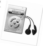
Ensure the MD has an input source for an external microphone, some newer models may not. In which case you will need an audio-buddy (*pre-amp*) into which the microphone links, that will then link to the MD recorder. Also ensure it has a digital output to connect digitally to a CD recorder.
