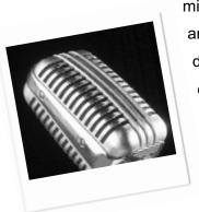
microphone is preferable if it is to be held when recording, as they are less susceptible to handling noise. These microphones, though, do pick up sounds coming from all directions, not just in the direction at which it is pointed. 19 Ensure all your equipment is compatible.
